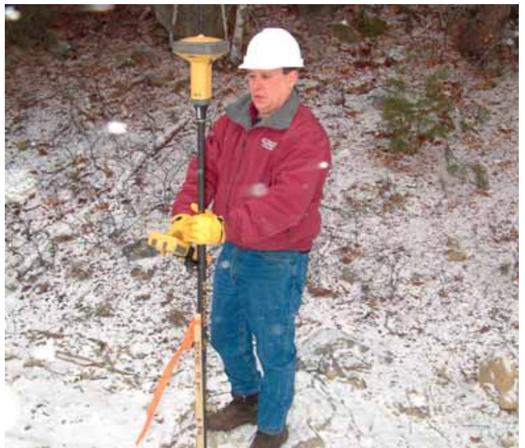
Steve Salsbury of Herrick & Salsbury sets up and uses the Topcon GR-3 RTK GNSS system and the FCS data collector
