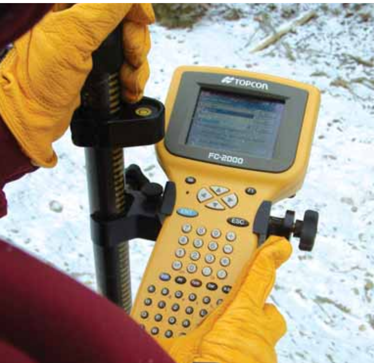
Steve Salsbury of Herrick & Salsbury sets up and uses the Topcon GR-3 RTK GNSS system and the FCS data collector
