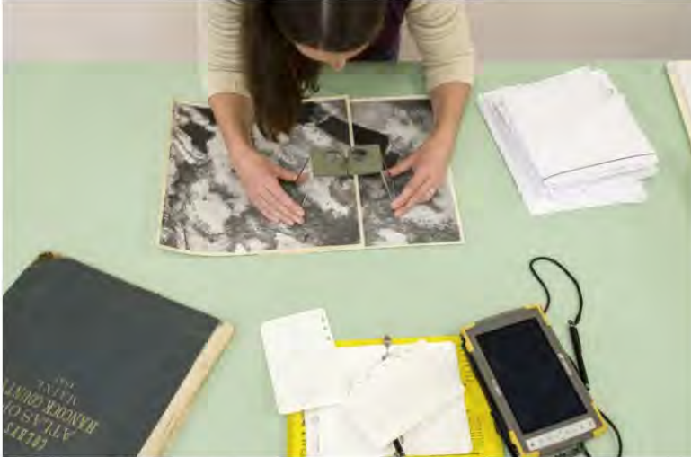
Ms. Hartson peering at aerial photos through a stereoscope for a three-dimensional view. Stacey Cramp for The New York Times
