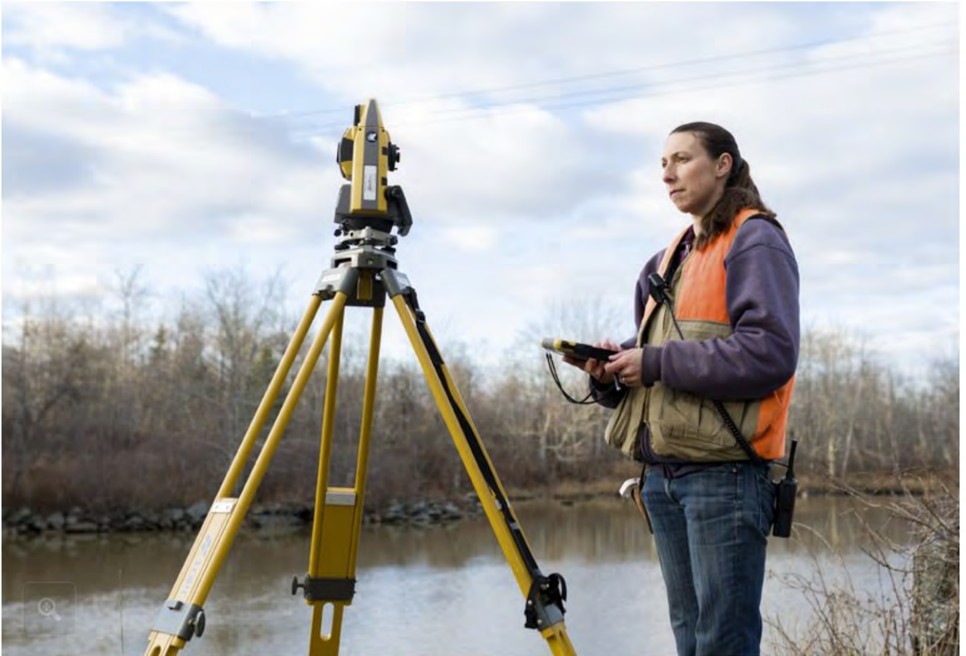
Tara Hartson, a surveyor at Herrick & Salsbury, using an instrument known as a total station, on the tripod, and a hand-held data collector to measure and record angles, distances and heights during a property survey. Stacey Cramp for The New York Times
