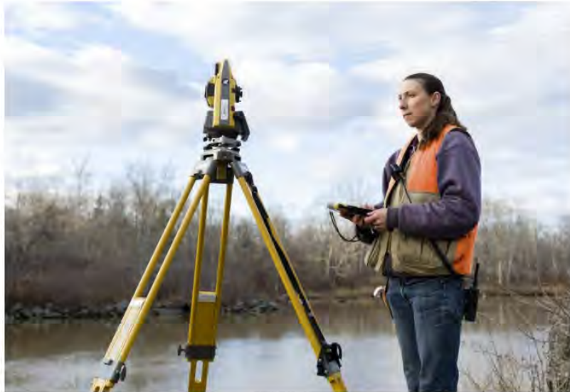
Tara Hartson, a surveyor at Herrick & Salsbury, using an instrument known as a total station, on the tripod, and a hand-held data collector to measure and record angles, distances and heights during a property survey. Stacey Cramp for The New York Times
